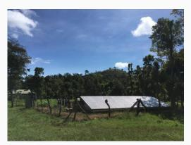
Under the water-collecting roof is a large pan. The water is pumped from here into the tank and irrigates the field.
